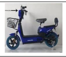
KS MODEL, 48V12AH Lead Acid Battery, 350W motor, drum brake, skd package
